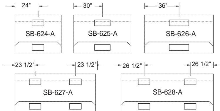
Duct collar locations are as shown above. The center line of each collar is 8" from the back of the hood. The center line of the supply duct is 35 5/8" from the back of the hood. The area indicated by the dashed lines is designated for plumbing and electrical rough-ins. All rough-ins should be kept within 7" of the wall and 18" from the floor.
