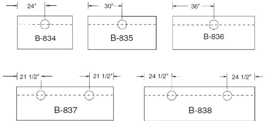
Duct collar locations are as shown above. The center line of each collar is 8" from the back of the hood. The area indicated by the dashed lines is designated for plumbing and electrical rough-ins. All rough-ins should be kept within 7" of the wall and 18" from the floor.
