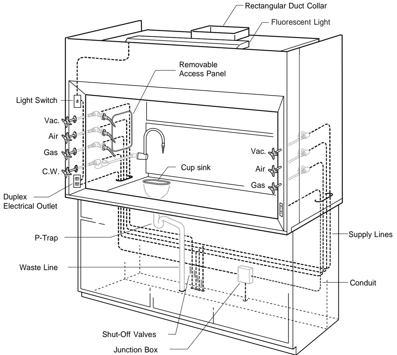
The above illustration depicts the routing of service and electrical lines in a typical Fume Hood. Unless specified otherwise, all service and electrical fixtures are shipped separately for installation in the field. Piping, conduit and wire are not included and must be furnished by others in accordance with local codes.
