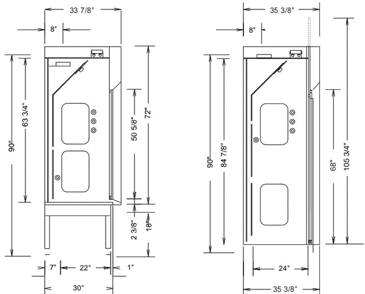
Duct collar locations are as shown above. The center line of each collar is 8" from the back of the hood.
