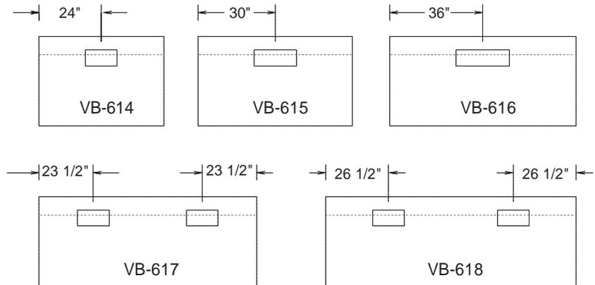
Duct collar locations are as shown above. The center line of each collar is 8" from the back of the hood. The area indicated by the dashed lines is designated for plumbing and electrical rough-ins. All rough-ins should be kept within 7" of the wall and 18" from the floor.
